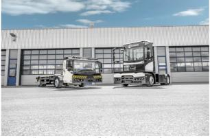
KAMAG "PrecisionMover" (PM) swap body transporter and "PrecisionTractor" (PT) terminal tractor.
