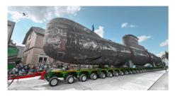
240 wheels roll U17 through the towns: An impressive sight at 350 tons, 48 meters long, and 9 meters high.
