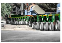
The axle compensation of the SCHEUERLE InterCombi vehicles helps with ballasting on the pontoon.
