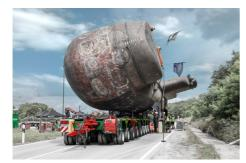
The world's first rotation of a submarine on a modular platform trailer
