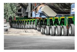
The axle compensation of the SCHEUERLE InterCombi vehicles helps with ballasting on the pontoon.
