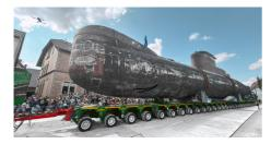
240 wheels roll U17 through the towns: An impressive sight at 350 tons, 48 meters long, and 9 meters high.
