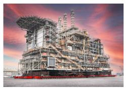
The introduction of SCHEUERLE SPMT technology revolutionised production. Since then, it has been possible to transport even gigantic components up to complete industrial and conveyor systems. Pictured: a 14,300-tonne oil and gas platform.
