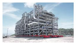
With the introduction of the SCHEUERLE SPMT in 2,430 mm width, transport undertakings could now take place even in the most remote places in the world. The container width enables fast, efficient and more costeffective transport of the SCHEUERLE SPMT modules in flat-rack containers.
