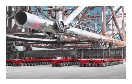
Whether coupled together or in an open network - there are no limits to the possible combinations of SCHEU-ERLE SPMTs. Thus, the payload is theoretically unlimited.
